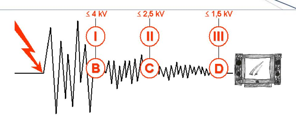
Lightning-currentSurge-voltageDarresterarresterproEN Type 1EN Type 2ENIEC Class IIEC Class IIIEC
